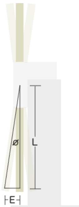
Illustration 2: Calculation of machine error from parameter RXX performed from the position of the mechanical rotation point.
