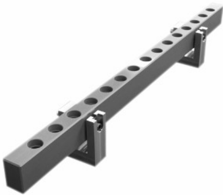
Illustration 5: Variation of a hole plate which is more like a ball bar. This is a 1D version of the 2D hole plate artifacts.
