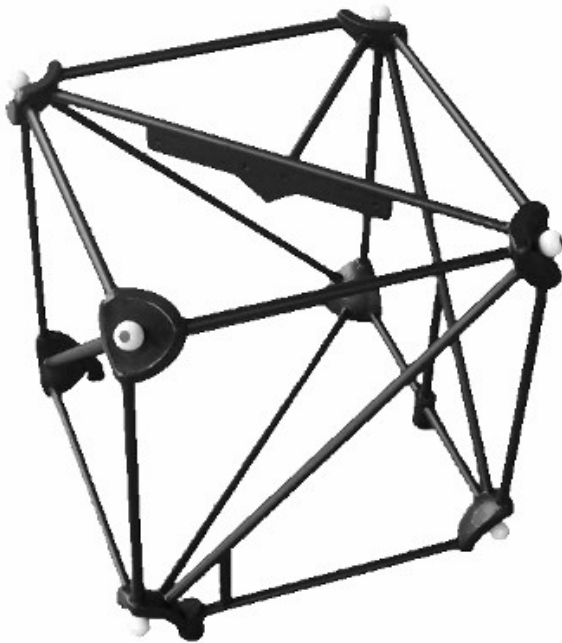
Illustration 6: Artifact used for volumetric testing
