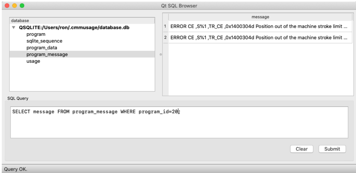
Illustration 2: Example of all error messages recorded for the program assigned to program_id of 20.
